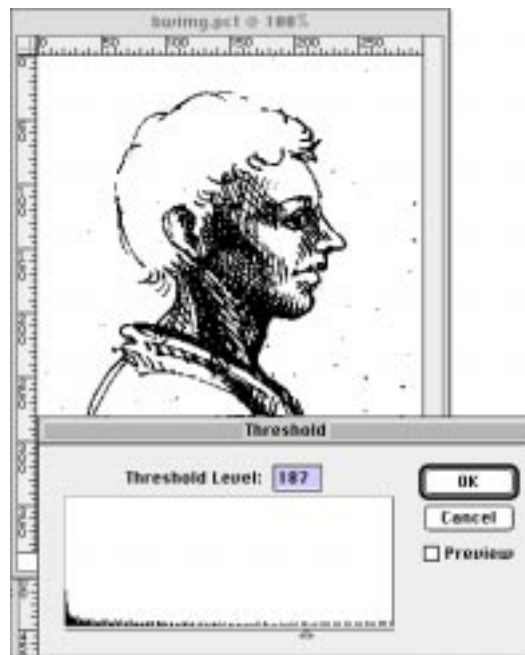
Figure 3: Setting a high threshold makes the image darker.
